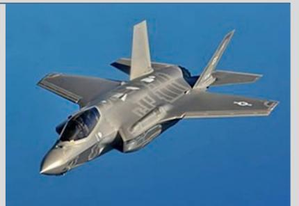
attack and air-superiority missions. The F-35 has three main variants: the conventional takeoff and landing F-35A, the short take-off and vertical-landing F-35B, and the catapult-assisted take-off but arrested recovery, carrier-based F-35C. For this EIS, the aircraft being considered is the F-35A variant.
